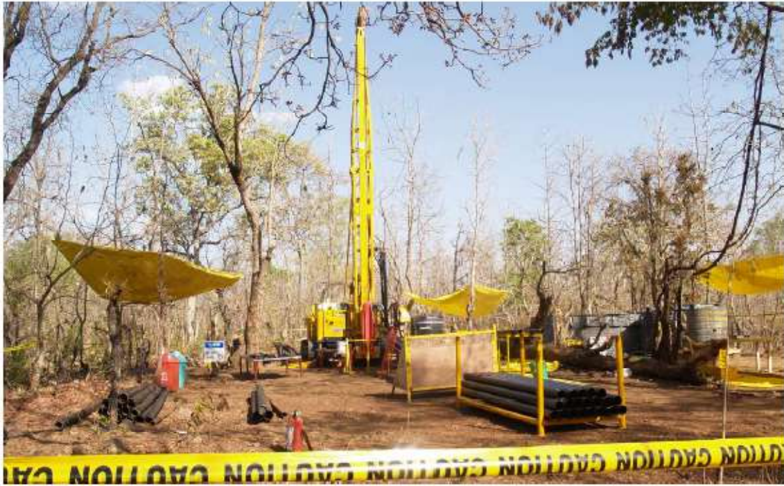
Figure 2 Drill Rig doing PQ drilling
