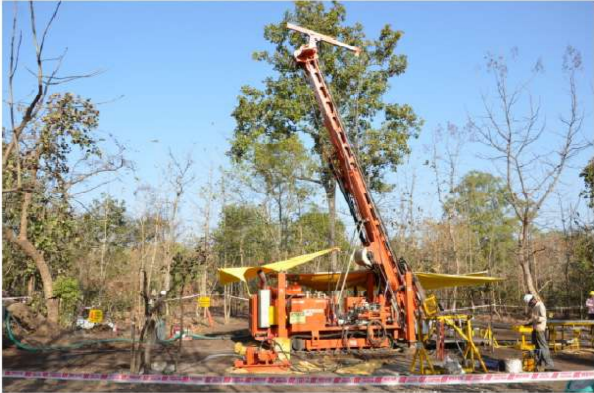
Figure 3 Drill rig doing HQ Delineation Drilling
